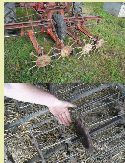
Top, the "Dixie," which can be used to cut weeds and thin crops. Below, the basket cultivator. The tractor operator must keep the crop in line between the baskets!
